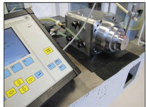
Fine tuning of balancing quality on the spindle
