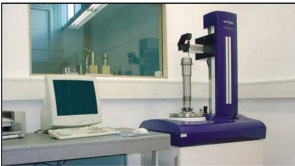
True-running gauging machine (to test rotation-symmetric parts of a spindle)
